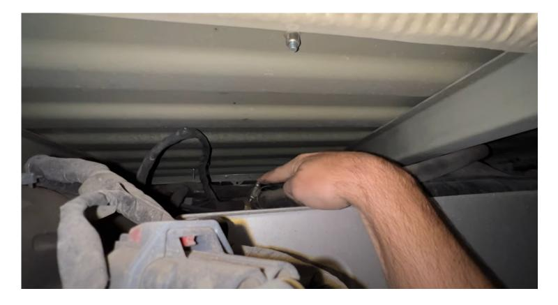
Remove the hose clamp and hose from the main vent line attached to the fuel sending unit. You can reach over the driveline to access this.
