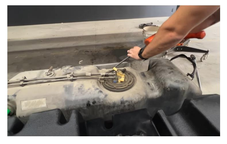
Hit the locking ring counter clockwise to release the OEM sending unit.
