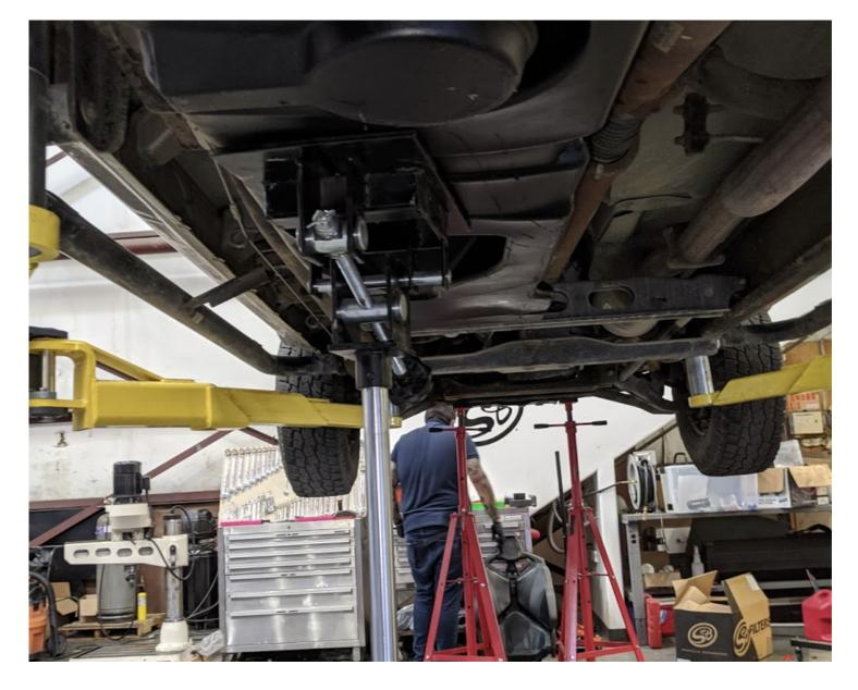
Center the hydraulic jack underneath the fuel tank and raise it into position. Lift Install: Hydraulic Jack Floor Install: Floor jack with added support to properly hold tank
