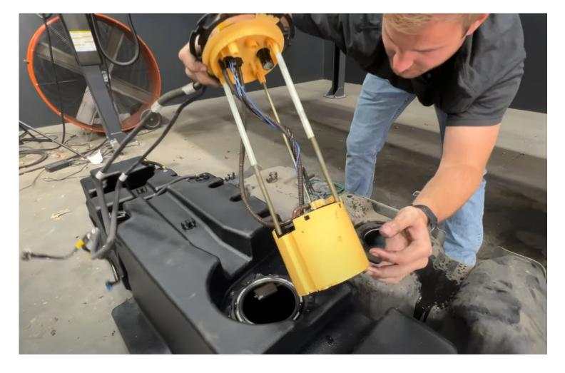
Place the included S&B oring in the oring groove on the S&B Tank. Install the sending unit and make sure to not damage the fuel float.
