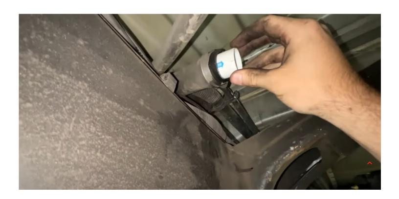
Place the included check valve into the filler hose. The arrow on the valve should be facing into the tank.
