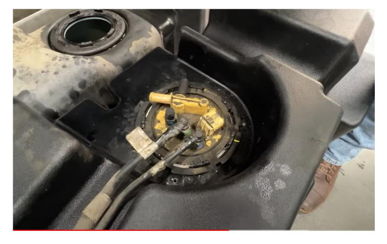
Press down of the locking ring to get the ring started and then hit the ring close wise until the locking ring goes under the indention in the ring and is locked into place.
