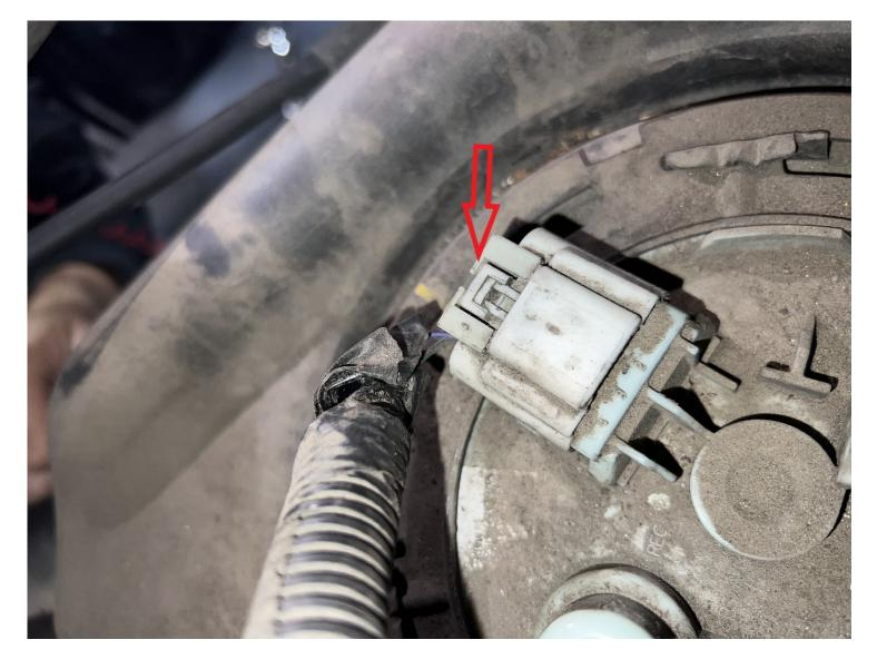
If you can reach the fuel sending unit electrical connector, you can disconnect it before dropping the tank. If you need more room to disconnect the connector, lower the tank 6" and disconnect. Slide the red lock out and depress the tab in the middle then slide the connector off.
