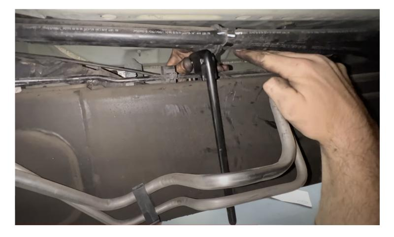
Install the included U-Bolt over the frame. Once installed, make sure there is space between the brake lines and U-Bolt. If the brake lines are touching the U-Bolt, call us and don't install the tank.
