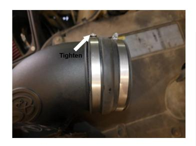
Insert the Intake Tube (A) first into the Intake Box (B) and then slide the other end of the Coupler (E) onto the turbo mouthpiece. Tighten the #72 Hose Clamp (U) on the turbo mouthpiece.
