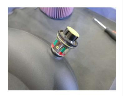
Install the Grommet Plug (T) into the Intake Tube (A).
