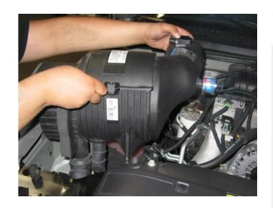
Remove the four bolts on the stock airbox tray and remove the tray from the vehicle. Be sure to save the speed clips underneath. They will be reused to install the Intake Box (B) in Step 9.
