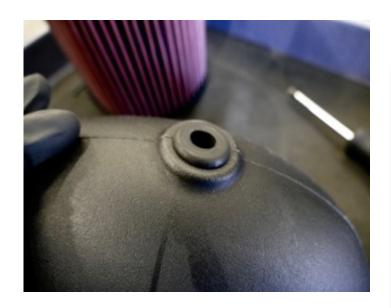
Insert the filter minder into the grommet.
