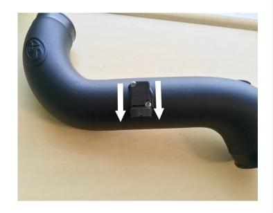
Insert the provided Grommet (P) into the Air Tube (L) if your vehicle came with a Filter Minder.
