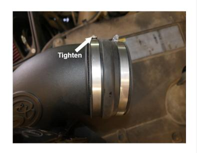
Insert the Air Tube (L) first into the Airbox (G) and then slide the other end of the Coupler (N) onto the turbo mouthpiece. Tighten the #72 Hose Clamp (M).
