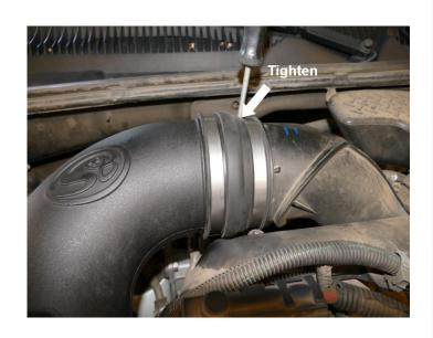
Slide the Air Filter (E) onto the Air Tube (L) and tighten the #80 Hose Clamp (F).
