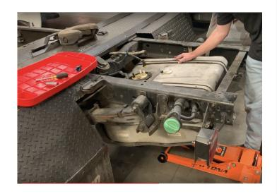
Clean the area around the fuel sending unit to prevent debris from getting into the tank when removing the sending unit. Now use a hammer and flathead screwdriver to remove the OEM sending unit. Position the screwdriver on a locking ring tab and hammer the unit counter clockwise. Once the locking ring is released, remove the sending unit.
