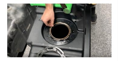
Now place your OEM sending unit in the S&B Tank. Make sure the knob on the sending unit is pointing towards the arrow molded into your S&B Tank. Be careful to not bend the float when installing the sending unit. Place the OEM locking ring on and hammer it clockwise.
