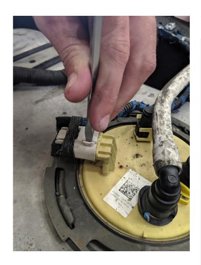
Slide the locking tab at the bottom of the fuel line connectors out. Be gentle as these connectors can become brittle with age.
