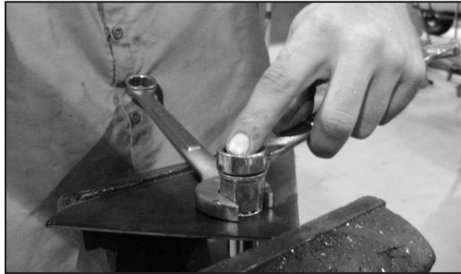
FIGURE 2 - 1/2" RIVET NUT SHOWN
